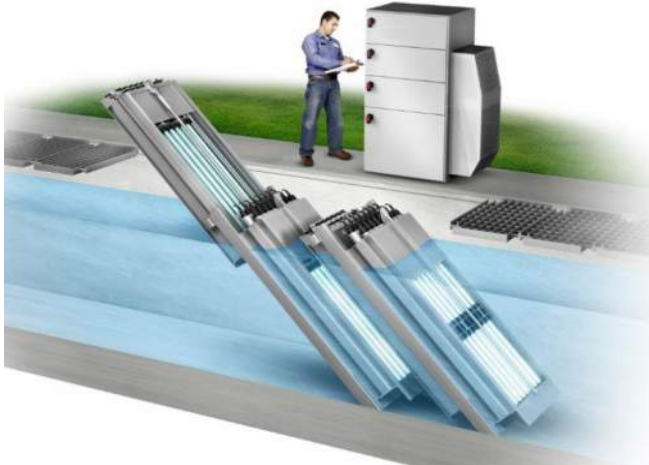
Figure 7-24: Ultraviolet Disinfection Illustration
