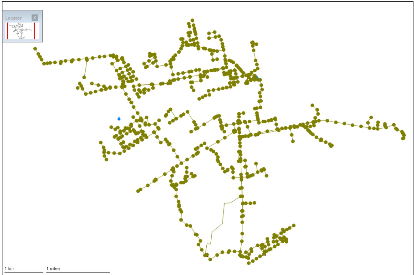
Figure 4-4: Sewer Collection System Hydraulic Model Skeleton
