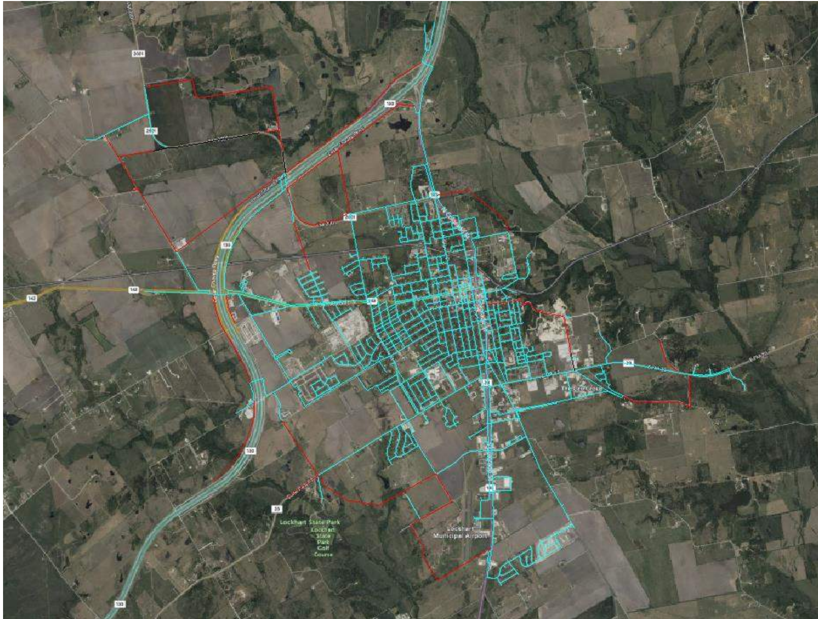
Figure 3-2: Water Distribution Hydraulic Model Skeleton
