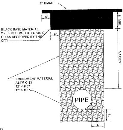
NOTE: UTILITY TRENCHES PLACED WITHIN THE STREET OR WITHIN 5' FROM BACK OF CURBS THAT ARE 3' OR MORE IN DEPTH SHALL COMPLY WITH THE R.O.W. DETAIL
